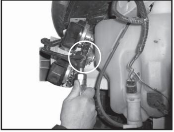
9. Remove one bolt from horn. Bolt will not be reused.
